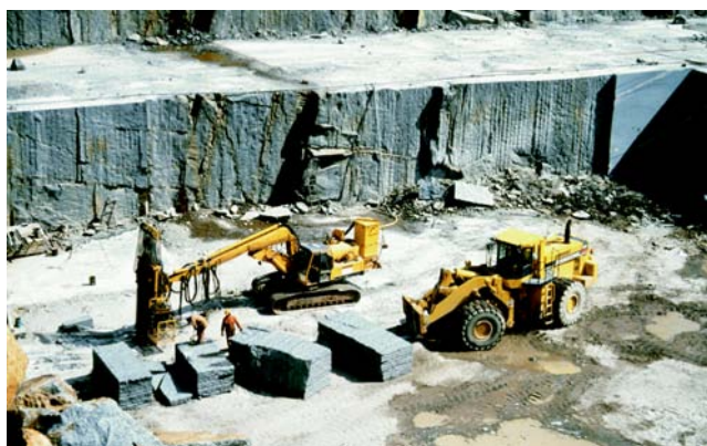
Fig. 2. Larvikite quarry, close to Larvik, Southeast Norway. A combination of drilling/blasting, diamond wire sawing and wedging is applied in the extraction process.
